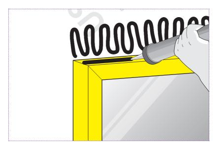
Apply Cortex Paste Adhesive to both the frame and the substrate using a paste adhesive gun.
