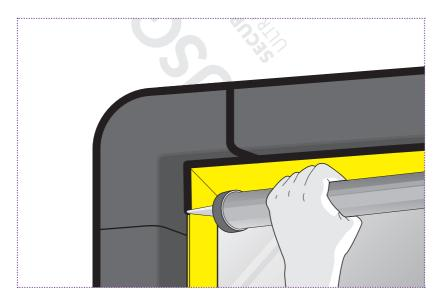
Corners can be sealed using Cortex 0901 External Corners. Apply a further bead of Cortex Paste Adhesive around the perimeter of the membrane and any joints/laps.
